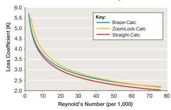
7/8" ACR Tube Loss Coefficient vs. Reynolds Number
